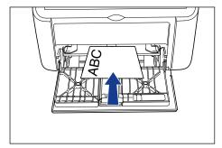
Slide the paper guides to fit both sides of the index card.
